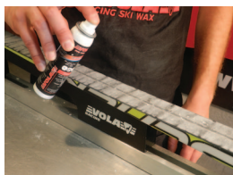
Application of WARM FINISHER between stages 3/ and 4/.
